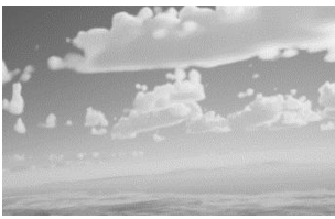
图 5 组合 CloudMap、高度相关函数以及形状噪声创建的云 Fig. 5 Cloud created by combining CloudMap, height dependent functions and shape noise
