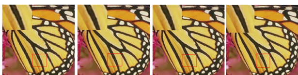
(e) DDSR (26.54 dB, 0.8886) (f) A+ (27.29 dB, 0.9092) (g) SRCNN (27.92 dB, 0.9245) (h) RDCR (27.60 dB, 0.9202)
