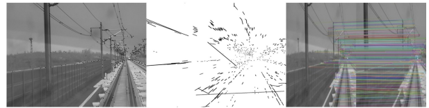
图 3 角点提取、轨迹及匹配图 Fig. 3 Corner extraction, trajectory and matching graph
