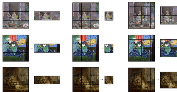
(a) Example of upper, middle, and lower blocks (b) Example of nine grid blocks (c) Example of overlapping blocks
