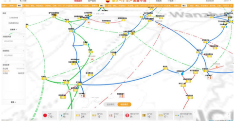
图 7 天然气智能调度计算机平台系统管网运行信息监控模块(地图监测) Fig. 7 Pipeline network operation information monitoring module of the natural gas intelligent scheduling computer platform system (map monitoring)
