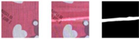
A fabric image of brown bear.pink background with Seam Pucker anomaly. The textile prints include white hearts and white polka dots. The heart pattern presents a dense arrangement.
