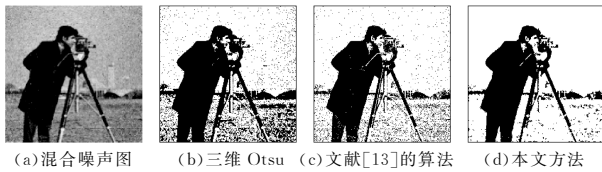
图 6 Cameraman 混合噪声的实验结果 Fig. 6 Results of Cameraman mixed with salt-and-pepper and Gaussian noise
